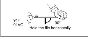
Important points for proper maintenance of saw chain:
